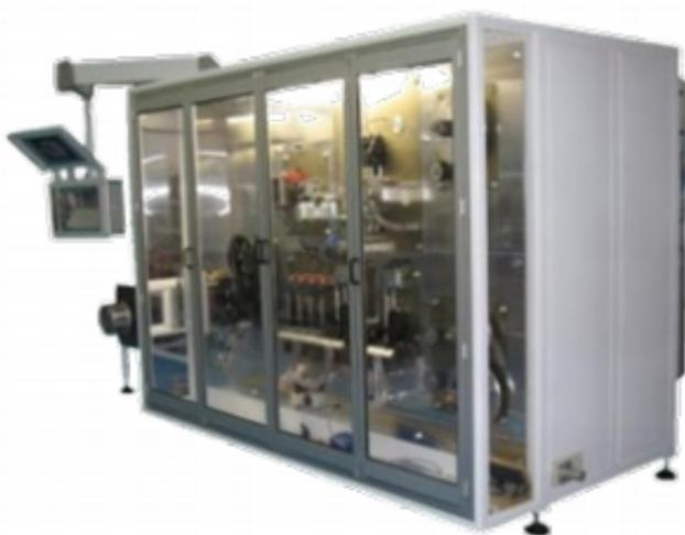
10 axis digital machine with 7 ultrasonic sealing systems
