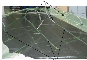
Resin transfer spiral (inside of vacuum bag)
