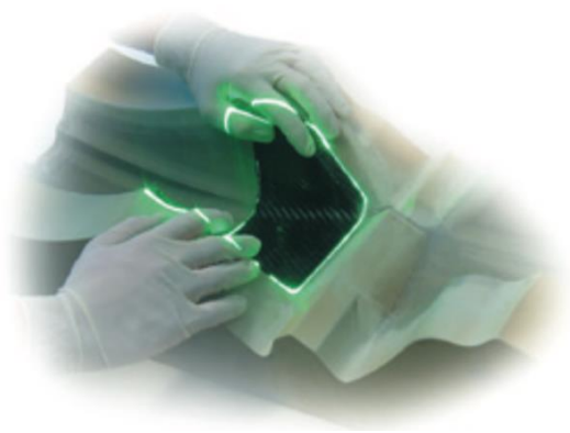
3D laser projection facilitates the positioning of prepregs
