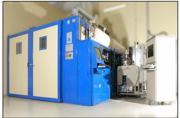
Oven: 3x4x2m, volume 24m 3 , Operating T=220°C
