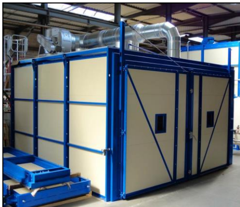
Oven: 5,5x6x3m, volume 99m 3 , Operating T=220°C
