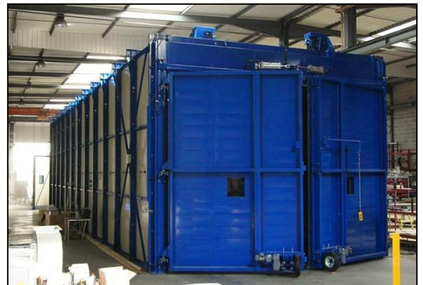
Oven: 6x22x4m, volume 528m 3 , Operating T=220°C
