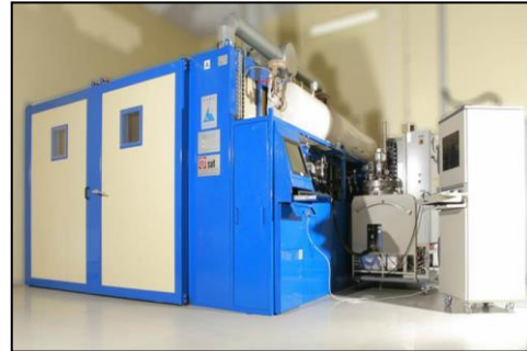
Oven: 3x4x2m, volume 24m 3 Operating T=220°C
