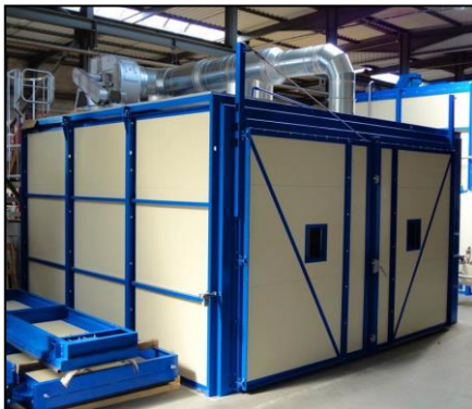
Oven: 5,5x6x3m, volume 99m 3 Operating T=220°C
