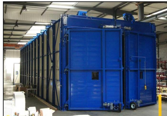
Oven: 6x22x4m, volume 528m 3 Operating T=220°C
