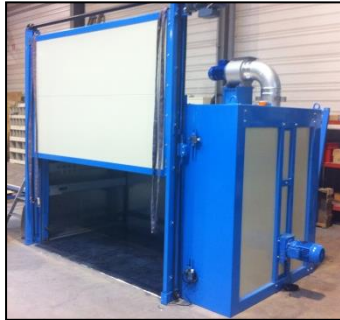
Oven: 2,1x1,1x1,3m, volume 3,00m 3 Operating T=250°C
