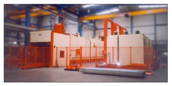
Standard volume of the furnaces with horizontal load: up to 30 m<sup>3</sup> (it is possible to increase the volume)
