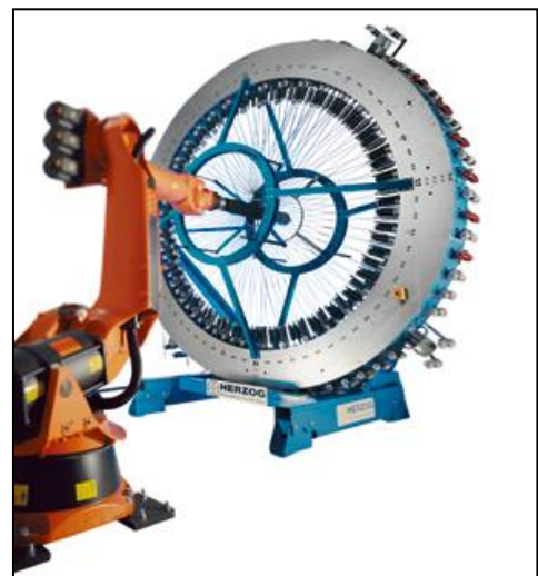
Radial braiding machine type with 144 carriers with multiaxial manipulator
