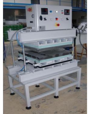
One regulation probe is connected in the platen. This probe is connected to the heating regulator and this regulator manage the heating cycle of each platen. Regulation with proportional approach (PID)
