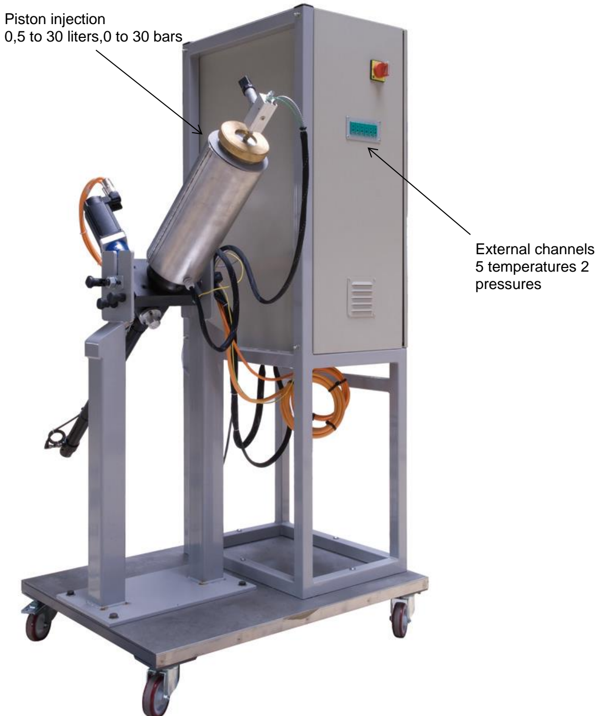
Picture 3: RTM Unit with PLC back side
