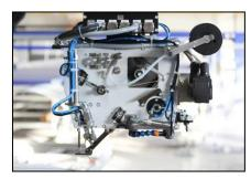
Single thread chain stitch seam is formed with one single needle thread, which is brought into the material by one curved needle from the top side of the material.
