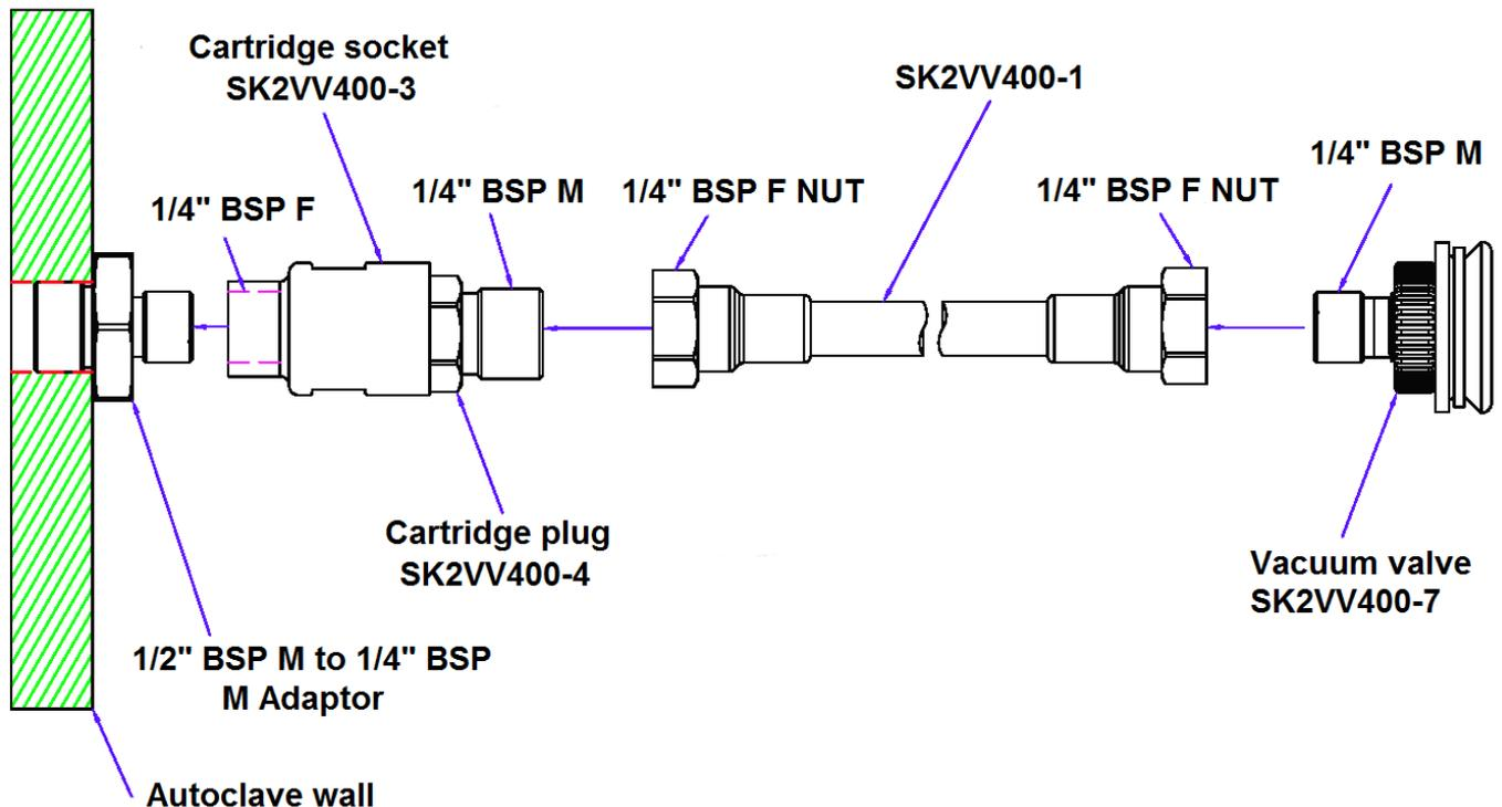
Assembling schema for using of super high temperature products for processes till 400°C
