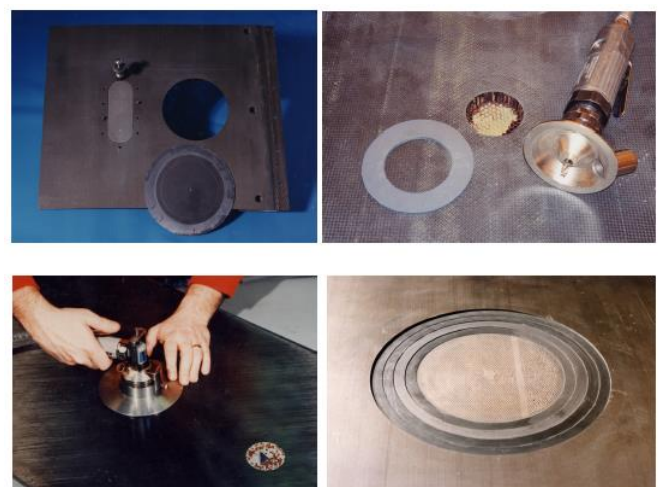
Photo 3: Routing, scarfing, stepping operations
