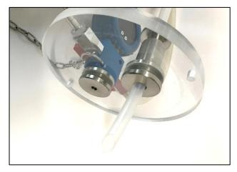
The trap is connected to the vacuum bag using the clamping fitting located on the transparent cover on the trap. This fitting is specially designed by VIK-COMPOSITE to prevent contamination by contact with the resin.
