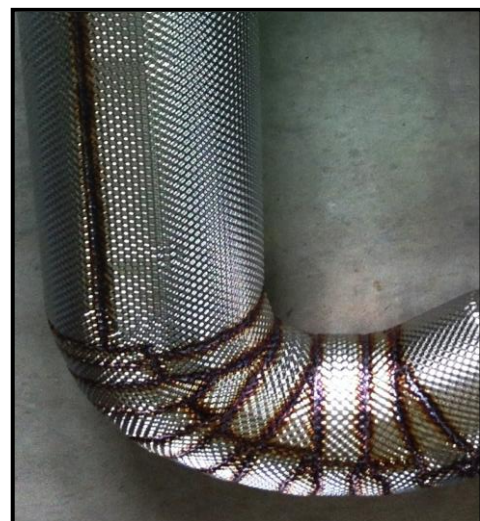
Mechanical engineering Foil: 0,15 mm Insulation: 20 mm
