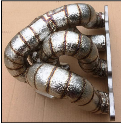
Manifold Foil: 0,15mm Insulation 6mm
