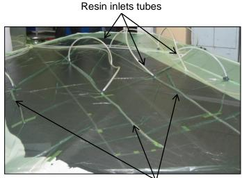
Resin transfer spiral (inside of vacuum bag)
