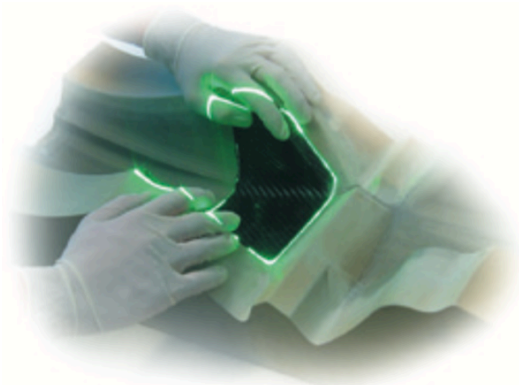
3D laser projection facilitates the positioning of preregs
