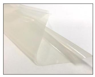
The silicone membrane is available in both cured SK2RS250-1 and SK2RS250-2 as uncured version. Cured material has a fine fabric impression to aid removal.
