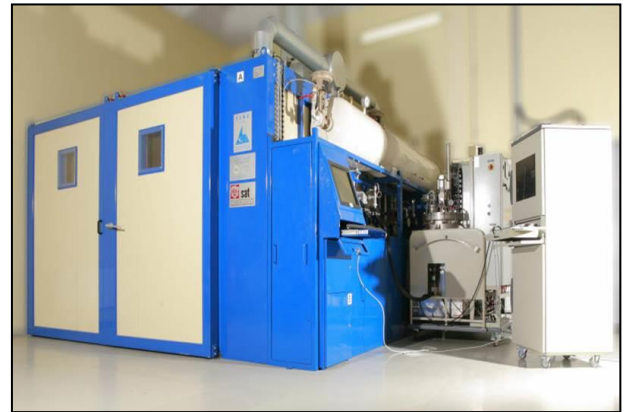
Oven: 3x4x2m, volume 24m 3 , Operating T=220°C
