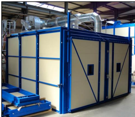
Oven: 5,5x6x3m, volume 99m 3 , Operating T=220°C
