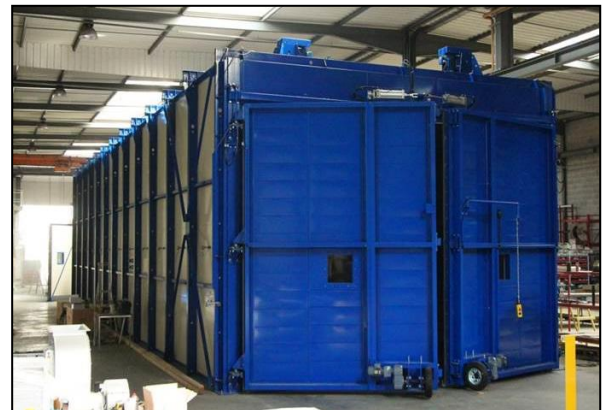
Oven: 6x22x4m, volume 528m 3 , Operating T=220°C
