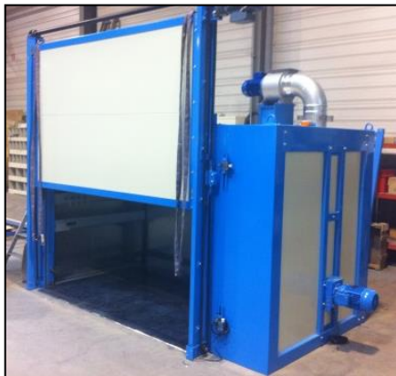
Oven: 2,1x1,1x1,3m, volume 3,00m 3 , Operating T=250°C
