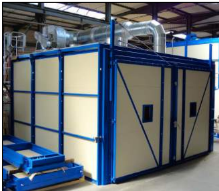
Oven: 5,5×6×3m, volume 99m 3 Operating T=220°C
