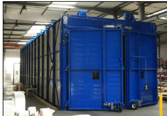
Oven: 6×22×4m, volume 528m 3 Operating T=220°C
