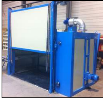
Oven: 2,1×1,1×1,3m, volume 3,00m 3 Operating T=250°C
