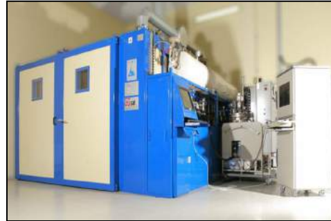
Oven: 3×4×2m, volume 24m 3 Operating T=220°C
