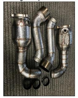
The components are wrapped with a special high-temperature-resistant mat and welded with embossed or spherical sheet metal. We work with a material thickness 4 to 10mm, whereby the total thickness - depending on the customer's wishes - could be adjusted by combining the thicknesses. Corrosion-resistant 1.4301 embossing foil is recommended for vehicles on the road, and temperature-resistant 1.4828 embossing foil for the racing segment.
