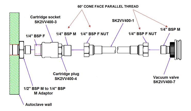
Assembling schema for using of super high temperature products for processes till  $400^{\circ}\mathrm{C}$
