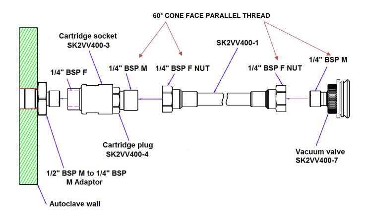
Assembling schema for using of super high temperature products for processes till 400°C
