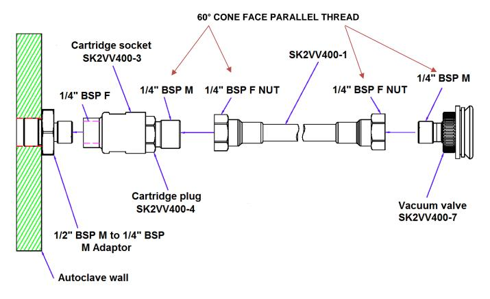
Assembling schema for using of super high temperature products for processes till  $400^{\circ}\mathrm{C}$
