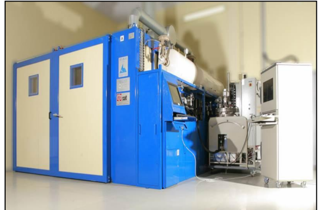
Oven: 3x4x2m, volume 24m 3 , Operating T=220°C
