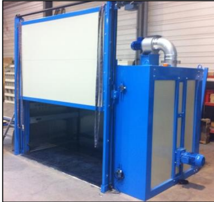
Oven: 2,1x1,1x1,3m, volume 3,00m 3 , Operating T=250°C
