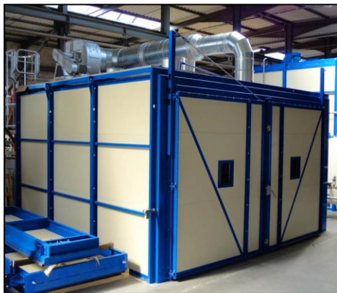
Oven: 5,5x6x3m, volume 99m 3 , Operating T=220°C
