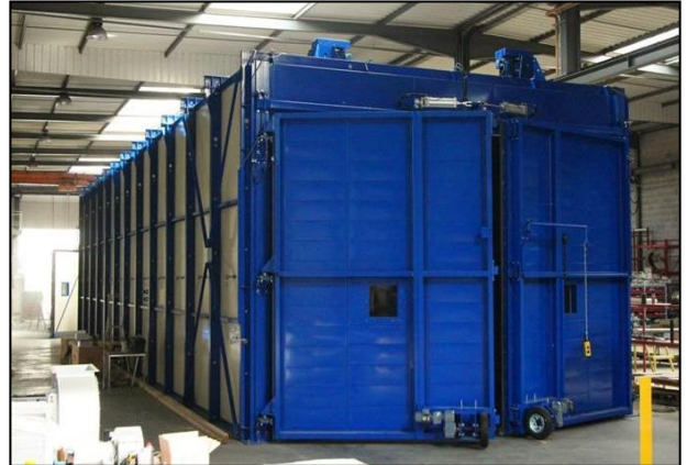
Oven: 6x22x4m, volume 528m 3 , Operating T=220°C
